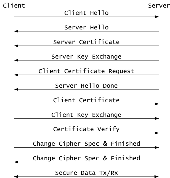
Fig. 2. Handshaking message exchange during secure communication establishment
